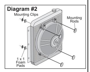
5. Cut off the excess Mounting Rods.
